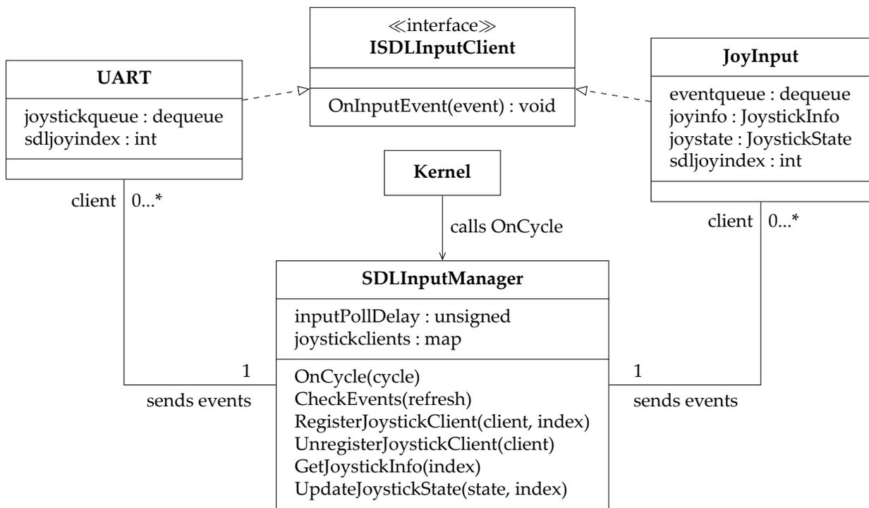
**Figure 4.1:** Simplified class diagram showing joystick related interaction
